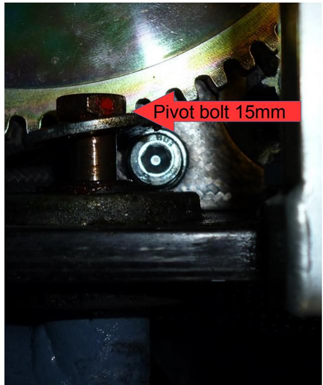
9. The head of the bolt on which the pylon pivots blocks removal of one starter motor bolt. Loosen pylon 17mm pivot bolt nut on the left side, then while holding nut with wrench, unscrew the pivot bolt just enough (careful here!) to let the starter bolt pass by.
