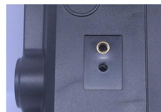
Press this switch for a few seconds to access setup. This switch is not accessible if the display is rotated (4.2), open the case for access.
