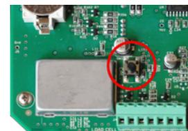
Press this switch for a few seconds to access setup.
