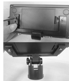
Install the **Support Part 2** on to the **Support Part 1** bracket (PT252 only) installed above as shown in the picture, after fitting the 2 Allen screws to it. **Support Part 2** can now be fitted over a round pole 38mm in diameter and locked in place with the Allen screws, or continue to the next step for mounting to a flat surface.
